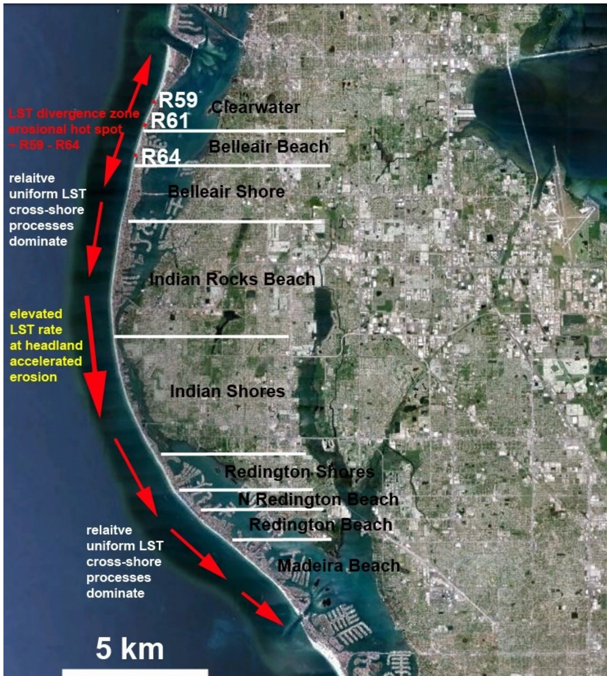
Figure 48: Generalized trend of net longshore sand transport along Sand Key and different beach segments.
